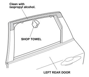
14. Peel back approximately 25–35 mm (1–1.5 inches) of adhesive backing, and tape the ends to the front surface of the left rear door visor.
