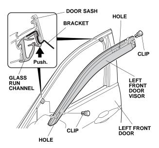
7. Align the door visor with the edge of the end cap.
