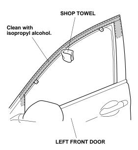
Peel back approximately 1½ to 2 inches of adhesive backing from each adhesive tape, and tape the ends to the front surface of the left front door visor with masking tape.
