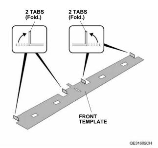
Line up the bottom of the template with the character line of the left front and rear doors, and line up the center hole of the template with the edge of the left front door. Then, attach the template to the left front and rear doors with masking tape as shown.
