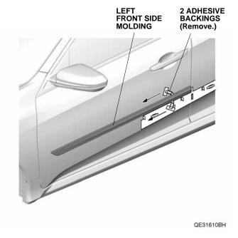
8. Using a rubber roller, apply firm pressure while rolling, especially at the ends, to set the adhesive.
