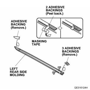
Line up the left rear side molding with the template and install the left rear side molding on the left rear door.
