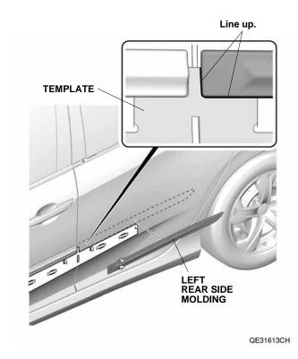
While applying light pressure against the left rear side molding, carefully remove the taped adhesive backings.
