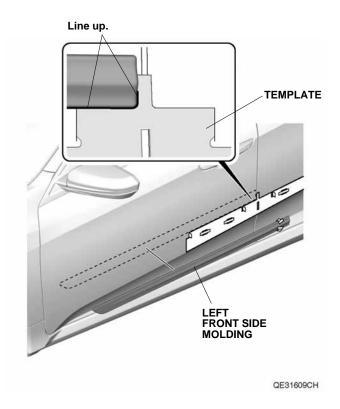
7. While applying light pressure against the left front side molding, carefully remove the taped adhesive backings.
