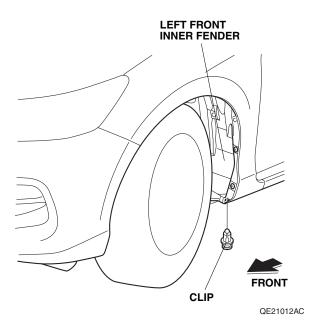
4. Install the left front splash guard to the left front inner fender in this order 1→2→3 using the two washer-screws and the clip removed in step 3. If necessary, trim the under sealant. Make sure there is no gap between the left front splash guard and the vehicle body. If there is a gap, loosen the three screws, hold the splash guard against the body, and tighten the three screws.
