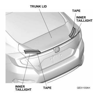
Place the template on the left side of the trunk lid, and align the template with the trunk lid as shown.
