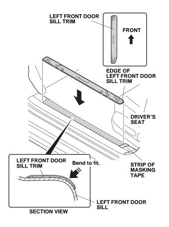
6. Using the palm of your hand, press the left front door sill trim firmly against the door sill, and remove the adhesive backing in the order shown. Apply firm pressure, especially at the ends.
