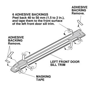
5. Starting at the curved area, bend the left front door sill trim against the left front door sill. Align the edge of the left front door sill trim with the masking tape, and install the left front door sill trim.
