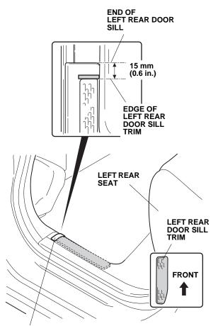
STRIP OF MASKING TAPE 3. Using one alcohol wipe, clean the front and rear door sills where the door sill trims will attach. Allow the alcohol to dry.
