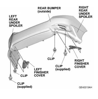
17. With the help of an assistant, install the rear bumper and left and right rear under spoilers with two hex bolts, four clips, and six self-tapping screws.
