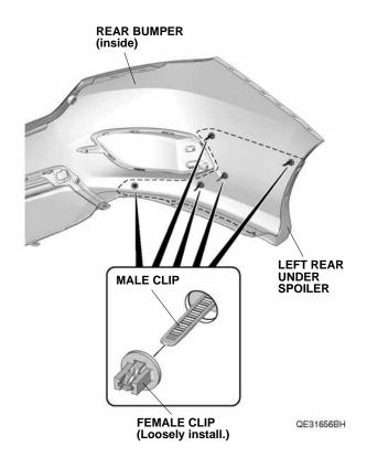
11. Remove three adhesive backings in the order shown. Press the left rear under spoiler firmly against the rear bumper with the palm of your hand.
