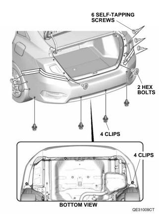
• With dual muffler: Remove two hex bolts, four clips, and six self-tapping screws.
