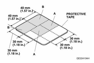
26. Apply masking tape to the vehicle panel as shown.
