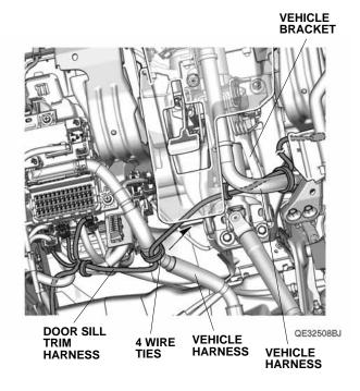
19. Secure the door sill trim harness to the vehicle duct with two wire ties.
