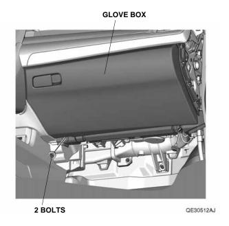
7. Open the glove box and remove the glove box.
