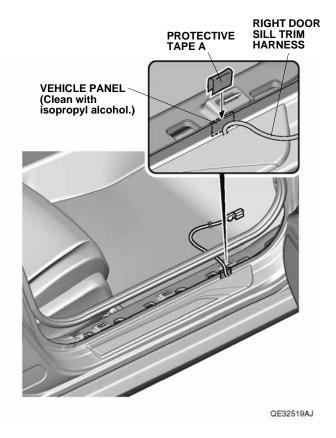
34. Install the protective clip to the protective tape A.
