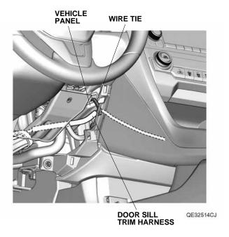
24. Route the door sill trim harness as shown. Secure the door sill trim harness to the vehicle harness with four wire ties.
