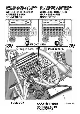
17. Attach the door sill trim harness 6-pin connector and fuse case to the vehicle connector.
