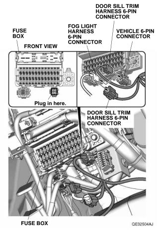
15. Plug the door sill trim harness 6-pin connector into the vehicle 6-pin connector. Go to step 17.
