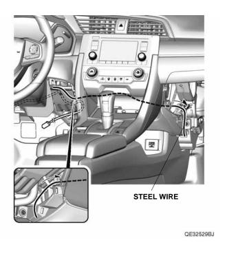
21. Attach the steel wire to the door sill trim harness with electrical tape.
