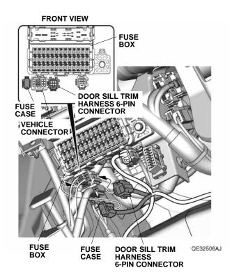
18. Route the door sill trim harness as shown. Secure the door sill trim harness to the vehicle harness and bracket with four wire ties.
