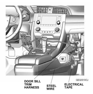
23. Secure the door sill trim harness to the vehicle panel with one wire tie.
