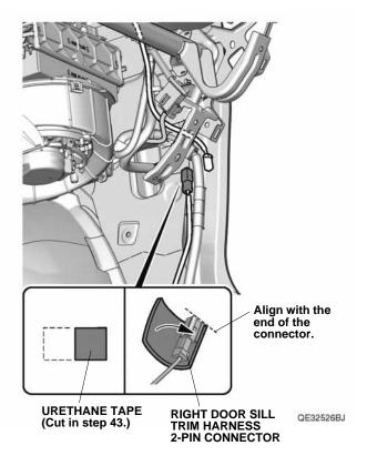
48. Plug the door sill trim harness 2-pin connector into the right door sill trim harness 2-pin connector.
