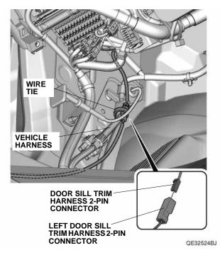
45. Secure the 2-pin connectors to the vehicle harness with one wire tie.
