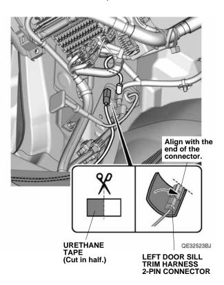
44. Plug the door sill trim harness 2-pin connector into the left door sill trim harness 2-pin connector.
