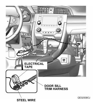
22. Route the door sill trim harness as shown and remove the electrical tape and steel wire.
