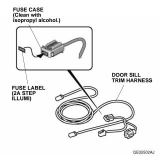
12. Attach the fuse label to the door sill trim harness fuse case.
