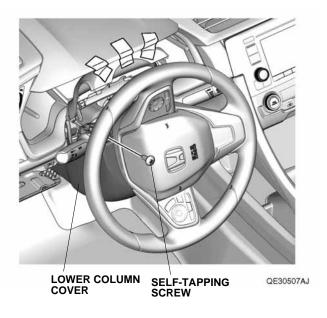
Turn the steering wheel 180° clockwise and remove one self-tapping screw from the lower column cover.
