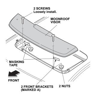
13. Install two screws through the two side brackets; then loosely install the nuts as shown. Remove the masking tape.
