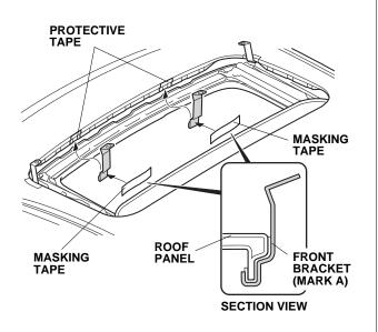
12. Set the moonroof visor on the vehicle roof in front of the moonroof opening, and adjust its position so the holes in the visor are aligned with the front bracket holes. Install two screws and nuts loosely into the front brackets. Remove the masking tape.
