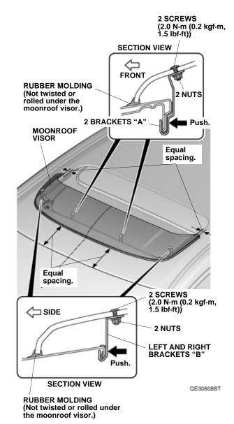
14. Tighten two screws and two nuts on the front of the vehicle first, then tighten two screws and two nuts on each side. Tighten while applying pressure so that there is no gap between the roof panel and the brackets "A" and "B". Torque the screws to 2.0 N·m (1.5 lbf·ft).
