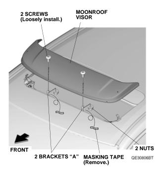
11. Loosely install the moonroof visor to the left and right brackets "B" with two screws and two nuts. Remove the masking tape from the left and right brackets "B".
