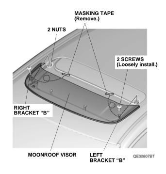
12. Check the information of the IMPORTANT INFORMATION label. To avoid wind noise, install the brackets against the body.
