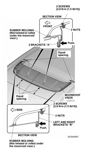
14. Tighten two screws and two nuts on the front of the vehicle first, then tighten two screws and two nuts on each side. Tighten while applying pressure so that there is no gap between the roof panel and the brackets "A" and "B". Torque the screws to 2.0 N·m (1.5 lbf·ft).
