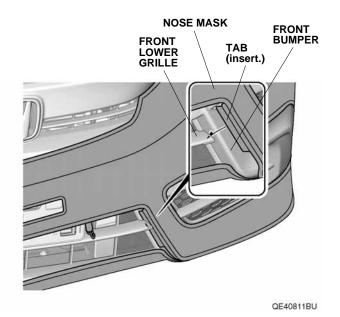
16. Attach three hooks and two S-hooks to the inside edge of the front lower grille opening as shown.
