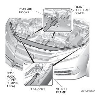
4. Attach the six hooks to the front grille opening. Insert the lower inner corner of the left tab between the front grille and front bumper, then push down and slide the tab until it's fully inserted between front grille and front bumper. Repeat for tab on the other side.
