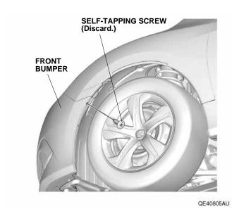
6. Install one snap-screw and one washer to the front bumper.
