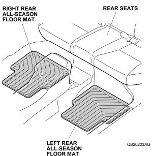
*2-Door:* Install the ring in the right rear all-season floor mat over the anchor. Push on the ring into the anchor to secure the retaining tabs, then turn the knob on the anchor 90° to secure the right rear all-season floor mat.
