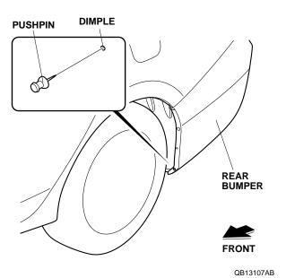
9. Pull away the rear bumper. Use a utility knife to cut the left rear inner fender in the area shown.
