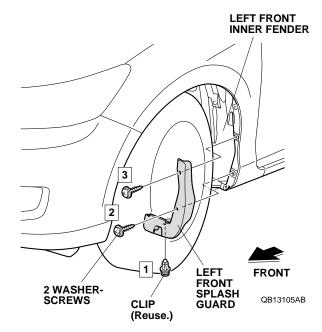
5. Turn the steering wheel fully clockwise, and repeat steps 2 through 4 to install the right front splash guard.
