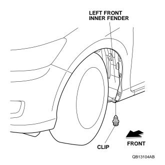
4. Install the left front splash guard to the left front inner fender with two washer-screws and the clip removed in step 3. Install the screws in this order
