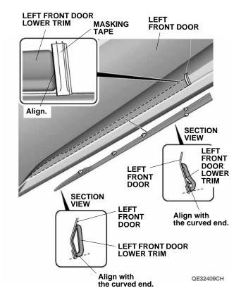
8. While applying light pressure against the left front door lower trim, carefully remove the taped adhesive backings.
