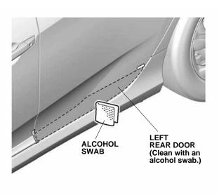
11. Peel back the adhesive backings and tape them to the front surface of the left rear door lower trim with masking tape. Remove the other adhesive backings.
