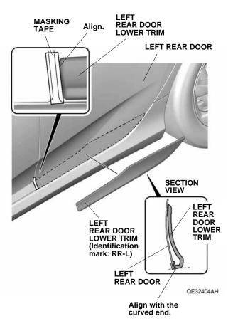
3. Apply masking tape to the left rear door as shown. Remove the left rear door lower trim.
