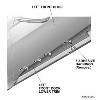
9. Using a rubber roller, apply firm pressure while rolling, especially at the ends, to set the adhesive.
