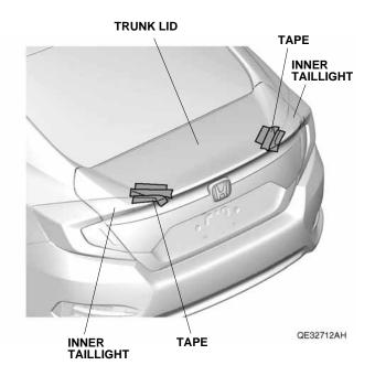
4. Place the template on the left side of the trunk lid, and align the template with the trunk lid as shown. Tape the template to the trunk lid with masking tape.
