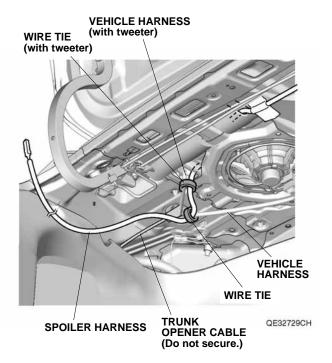
32. Plug the spoiler harness 2-pin connector into the wing spoiler harness 2-pin connector.
