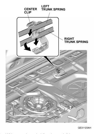
23. With an assistant holding the trunk lid open, remove the right trunk spring from the slider using the trunk spring tool. Wear gloves to protect your hands, and push down on the trunk spring tool slowly and carefully.
