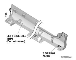
11. Install the three spring nuts on the left spoiler.
