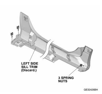
11. Install the three spring nuts on the side under spoiler as shown.
