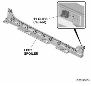
13. Install the left spoiler on the vehicle panel.
