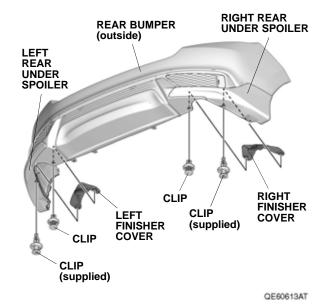
17. With the help of an assistant, install the rear bumper and left and right rear under spoilers with two hex bolts, four clips, and four self-tapping screws.
