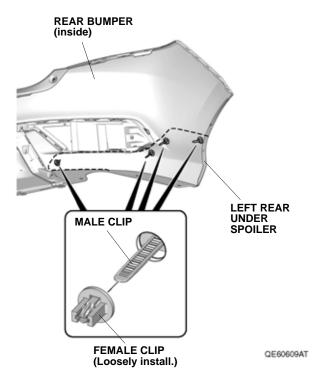
11. Remove two adhesive backings in the order shown. Press the left rear under spoiler firmly against the rear bumper with the palm of your hand. NOTE: Make sure there is no gap between the left rear under spoiler and the rear bumper
