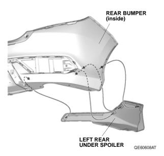
10. Loosely install four female clips into each of the male clips.
