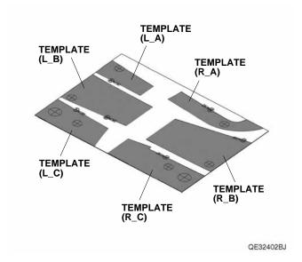
15. Attach the templates to the left lower trim with masking tape.
