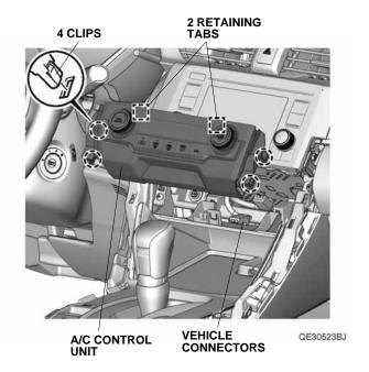
9. Remove the shift lever console panel:
