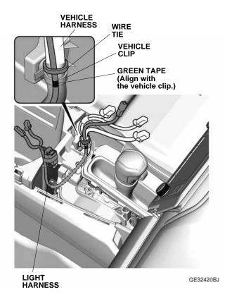
45. Secure the light harness 2-pin connector to the vehicle harness with one wire tie.
