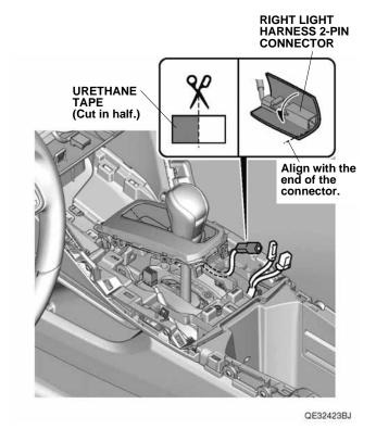
48. Using scissors, cut one urethane tape in half, and attach one piece of urethane tape around the right light harness 2-pin connector.
