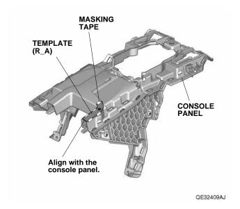
28. Using a pushpin, pierce the center of the mark on the template.
