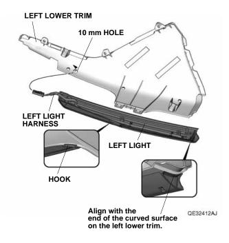
33. Secure the left light to the left lower trim with three self-tapping screws.
