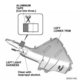
35. Using scissors, cut one aluminum tape into three pieces, secure the left light harness to the left lower trim with one of the pieces of aluminum tape.
