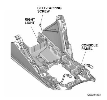
41. Secure the right light to the console panel with one self-tapping screw.
